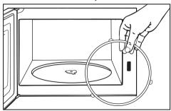
Always keep the roller ring underneath it clean as well as the oven floor to enable the turntable to turn smoothly. ■ Clean the surfaces between the turntable and the roller ring.
